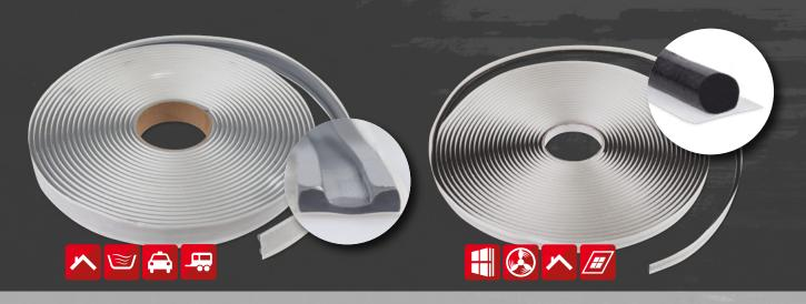
Butyl tape B1 and B1+ – butyl laminated with fleece, adhesive on one side, protected with paper or film. The B1+ version is additionally equipped with an acrylic self-adhesive strip. Standard sizes: 75, 100, 150 mm. **Butyl tape B2** – butyl coated with aluminium film (pure or laminate), adhesive on one side, protected with paper or film. **Standard sizes: 50, 70, 100, 150 mm.**
