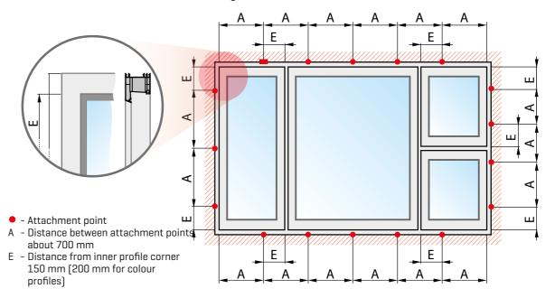
Diagram of window and door support taking into account forces acting on the window plane (weight of the window and operating load)
